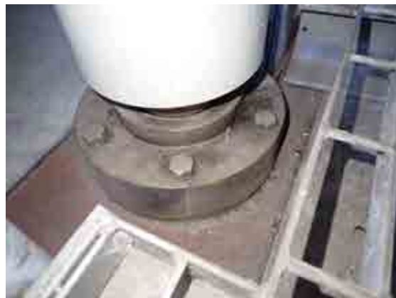
Right side central casing support foundation.
