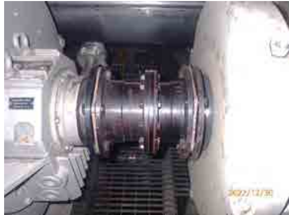
Flexible coupling overall condition.
