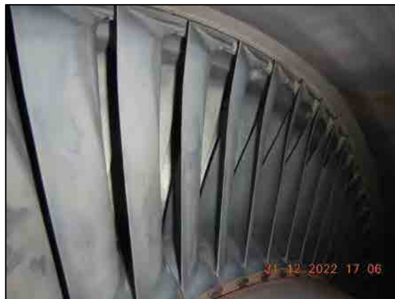
Turbine blades stage 3 trailing edge overall condition.
