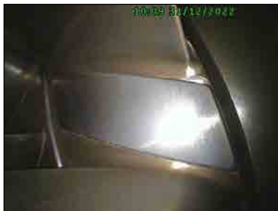
Compressor rotor stage 6 condition
