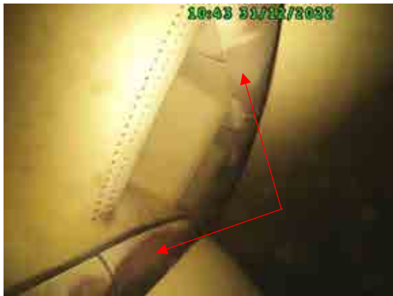
Inner/Outer vane plate condition at burner position 15.
