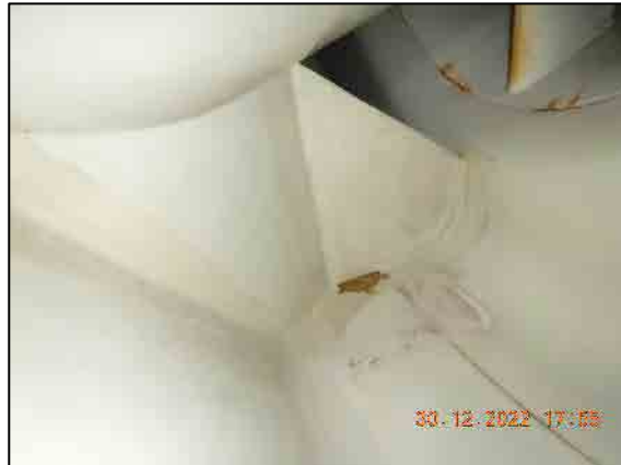
Example of compressor wash spray nozzle condition. Inlet casing drain port overall condition.
