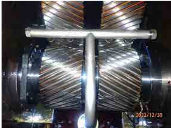
Pinion cogs condition.
