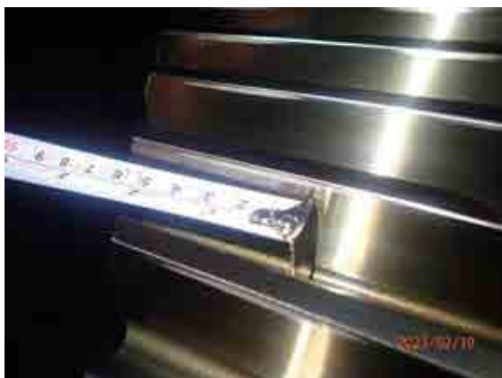
White mark 3.0 cm at left side on left wheel.
