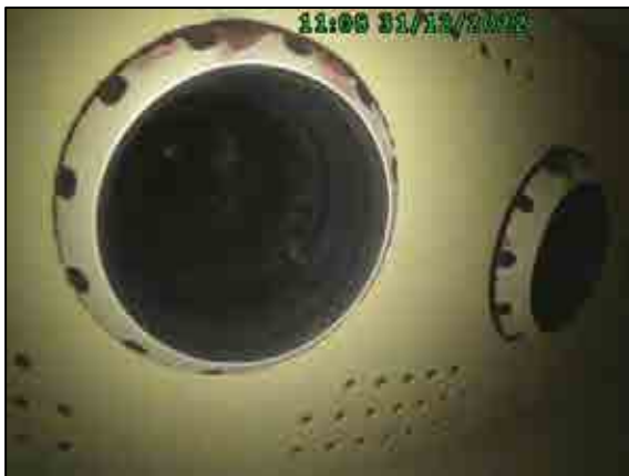
Example of close-up burner condition on front panel. Inner/outer wall TBC condition between GV1 entrance.
