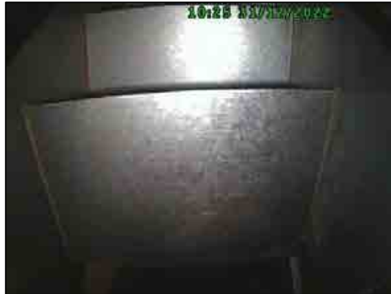
Compressor guide vanes stage 10.
