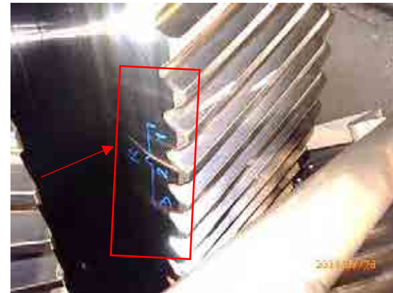
Electro static discharge 15 cm at left and right side on right wheel and follow up location at next inspection
