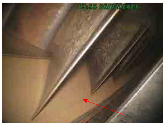
Abradable seal stage 11 condition.
