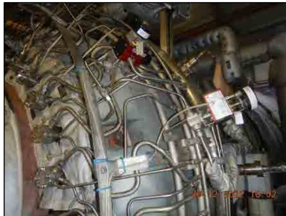
Ignition control valves overall condition.
