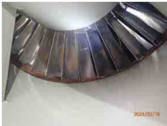
Compressor Inlet guide vanes stage 0.
