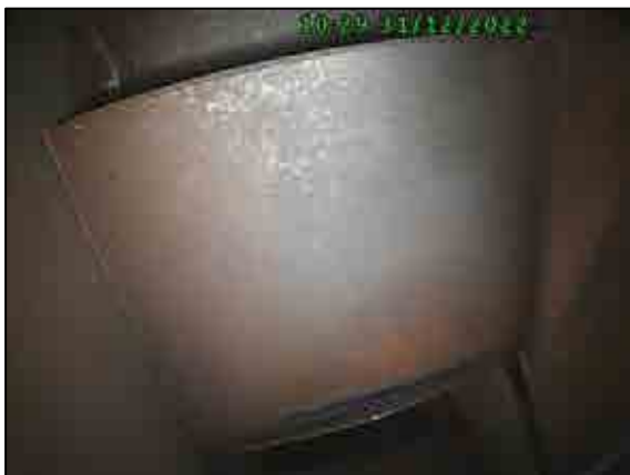
Compressor guide vanes stage 13.
