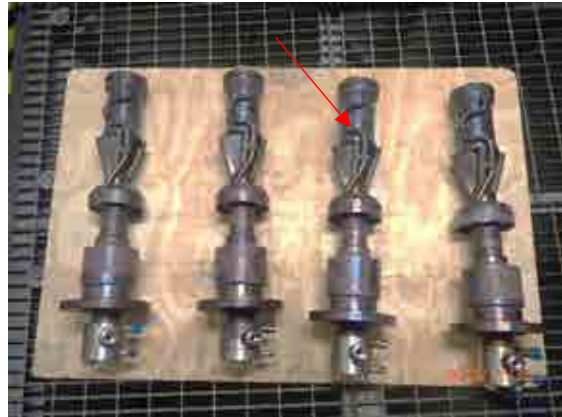
Dismantled burner#7 overall condition.
