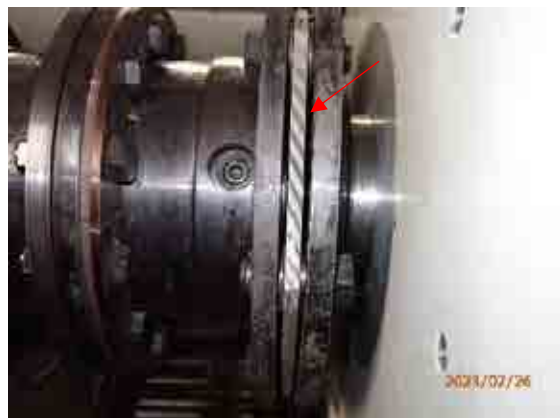
Flex plate bundle condition on gearbox side.
