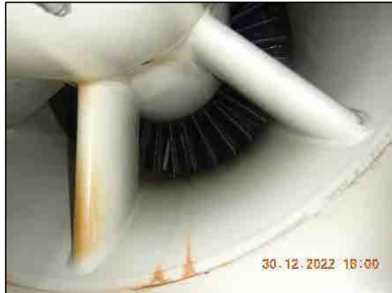
Right side dirty water trace condition.
