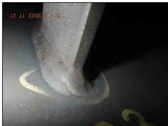
Example crack found at this area.
