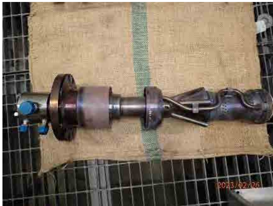
Dismantled burner#22 overall condition.
