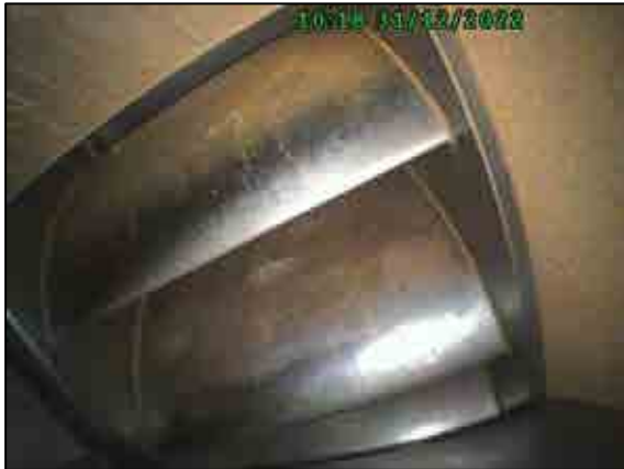
Compressor guide vanes stage 9.
