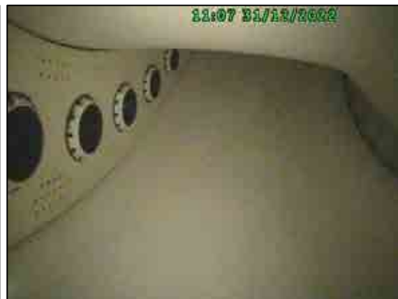
Inner/outer wall TBC condition, different location.
