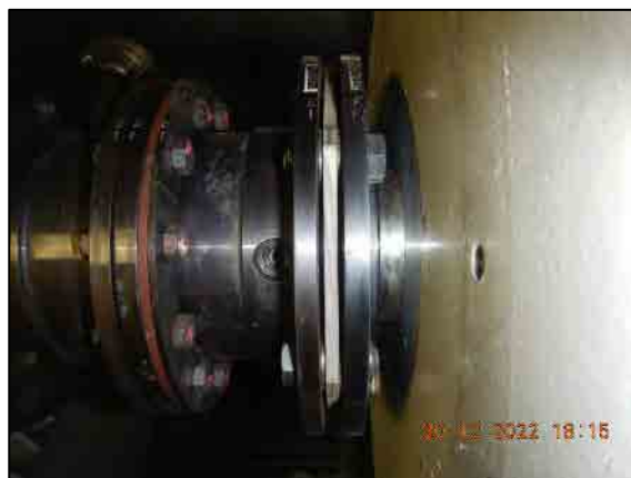
Shim pack separation condition on gearbox side.
