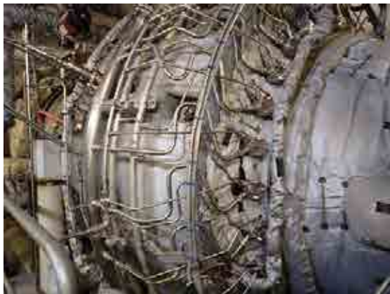
Manifold ring supply to burners overall condition.
