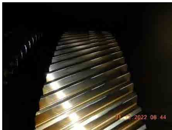
Wheel non-active side white mark (Turbine side).
