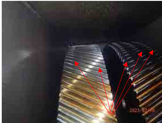
Wheel gear condition found white mark
