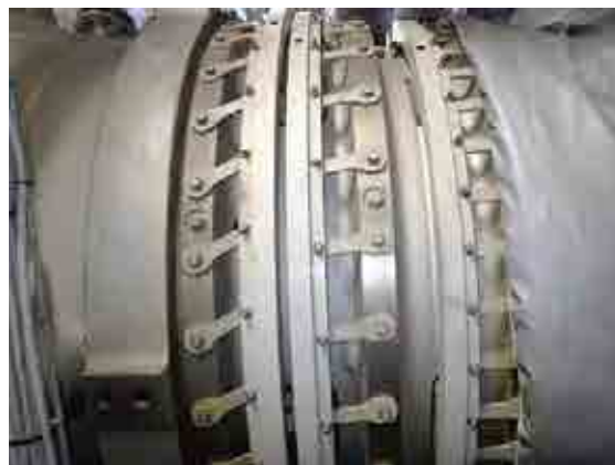
GV actuator mechanism overall condition right side.
