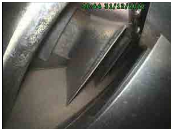
Compressor blades stage 12 condition.
