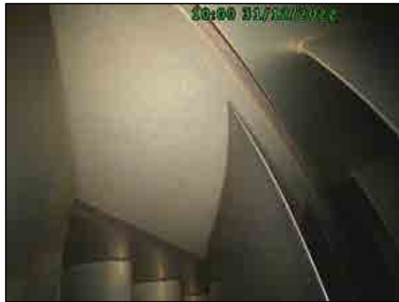
Abradable seal stage 4 condition.
