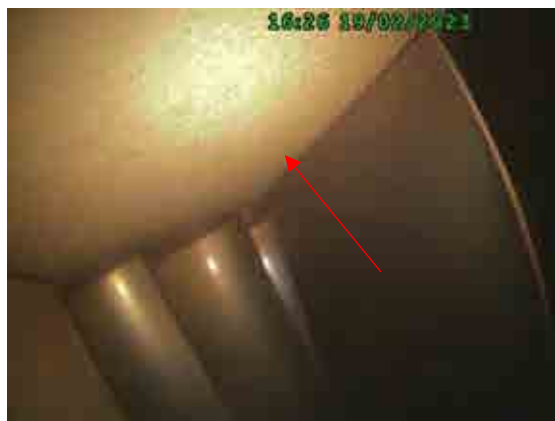
Abradable seal stage 5 condition.
