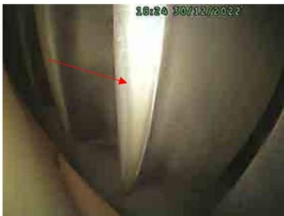
Turbine blades 2 leading edge condition.
