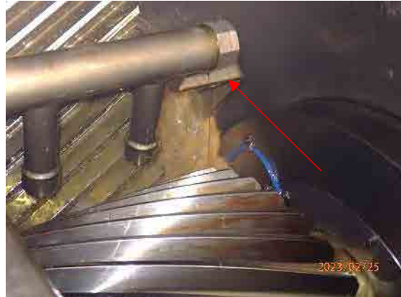
Oil leakage on right side of manifold.
