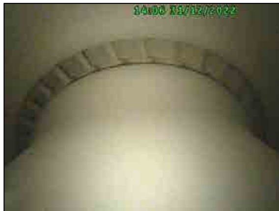
Example of close-up burner condition on front panel. Inner/outer wall TBC condition between GV1 entrance.
