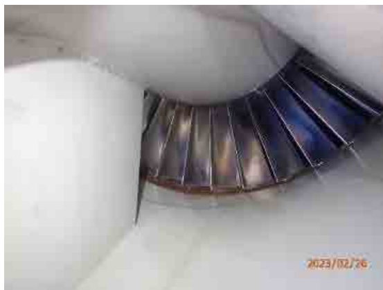
Compressor Inlet guide vanes stage 0.
