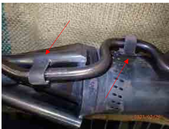
Gas fuel wings and pilot fuel pipe overall condition.
