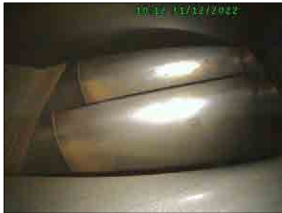
Compressor guide vanes stage 6.
