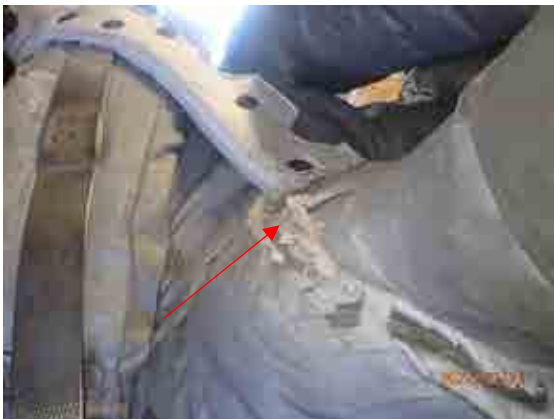
Condition of insulation on bleed pipe.
