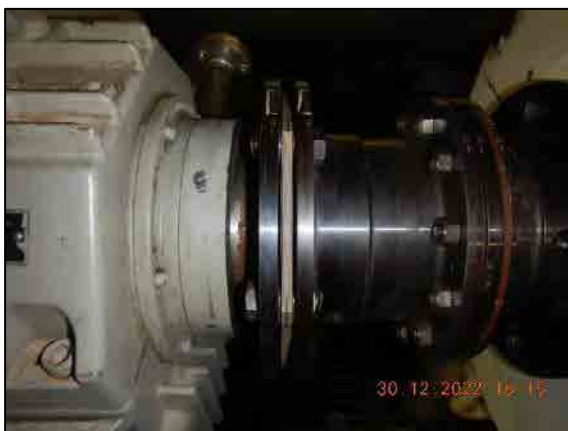
Shim pack separation condition on stator motor side.
