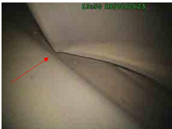
Condition leading edge tip blades 3.
