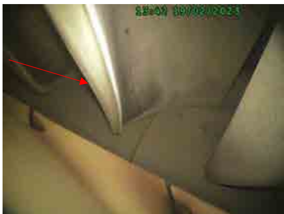
Turbine blades 2 leading edge condition.
