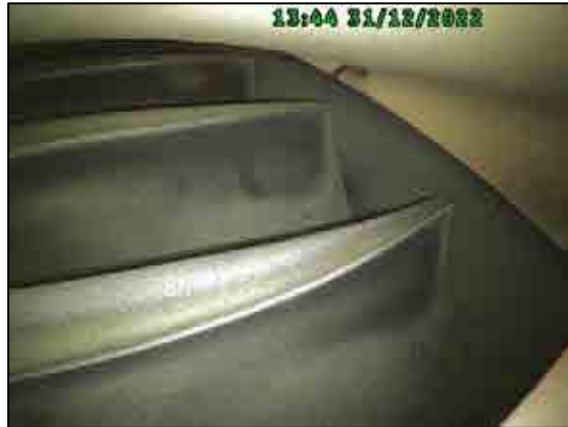
Leading edge tip condition of turbine blades stage 2.
