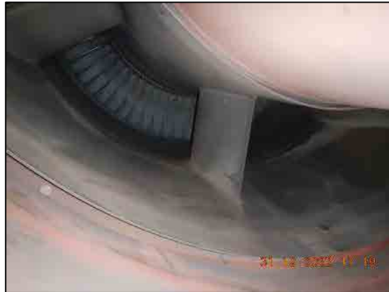
Inner/outer heatshield and struts right bottom condition.
