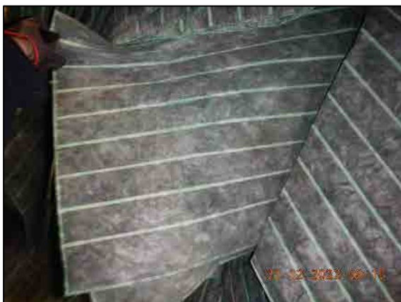
Example of pre-filter contamination condition.
