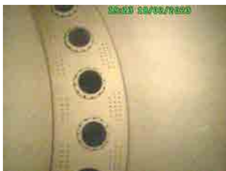
Front panel with burners from burner#1.
