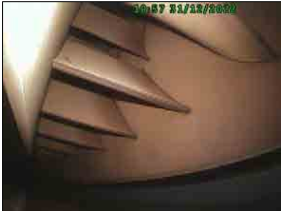
Compressor guide vane stage 15.
