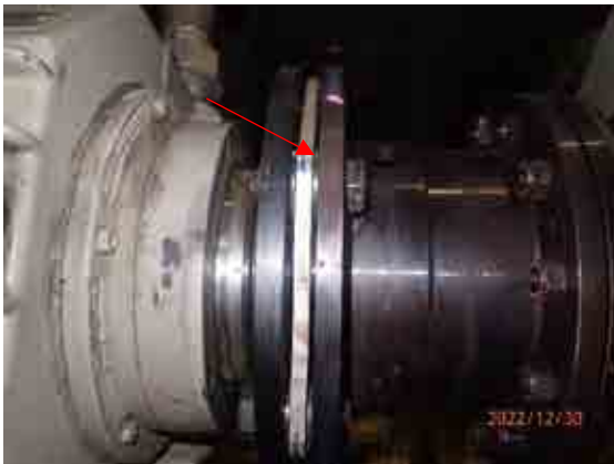
Flex plate bundle condition on starter motor side.
