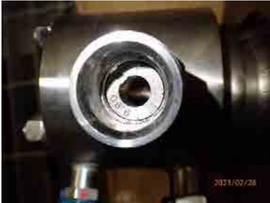
No yellow powder deposit in main gas fuel.
