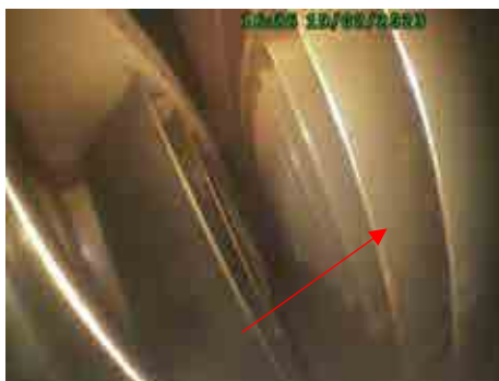
Compressor guide vanes stage 5
