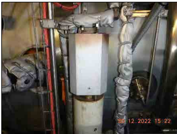
Left central casing support pendulum.
