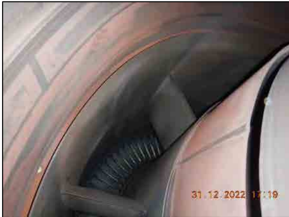
Inner/outer heatshield and struts right condition.
