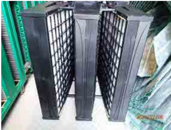
Fine filter as found condition.
