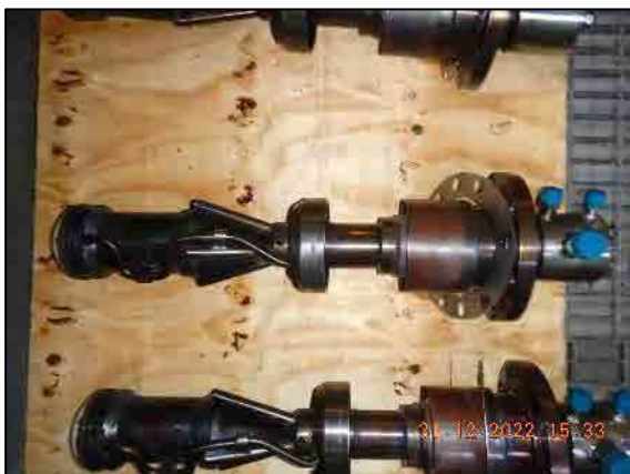
Overall condition of burner#1.
