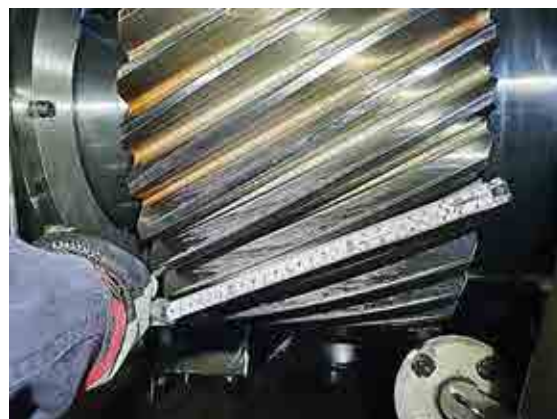
White mark on pinion gear gas turbine side.
