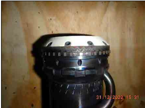
Condition of TBC coating at pilot flame nozzle.
