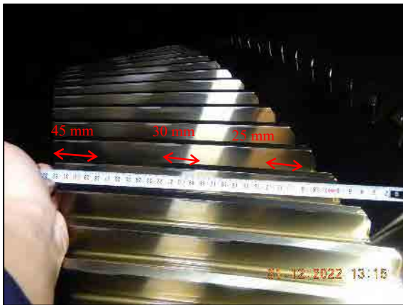
Recorded white mark on wheel cogs generator side. Recorded white mark on wheel cogs turbine side.
