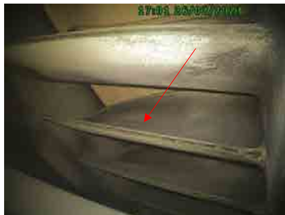
Turbine blades 2 trailing edge cooling passages.
