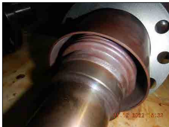
Outer bellow overall condition.
