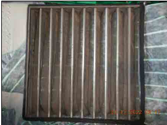
Intake side condition of pre-filter element.
