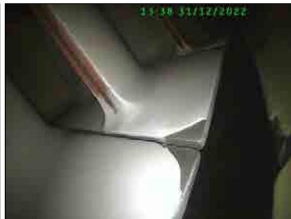
Example of blade 1 trailing edge base platform condition.
