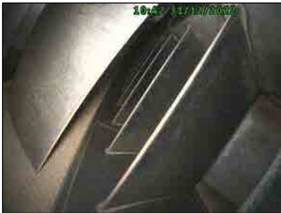
Compressor guide vanes stage 11.
