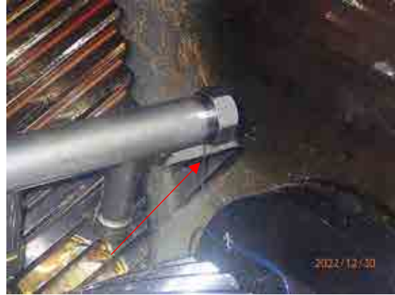
Lube oil leakage at end cap right side of manifold
