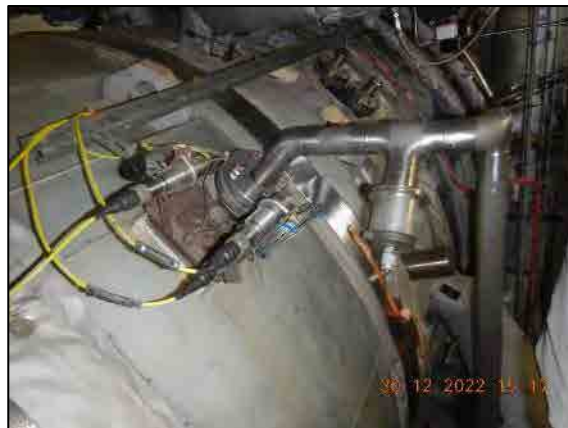
Lube oil supply to bearing 2 flange overall condition.
