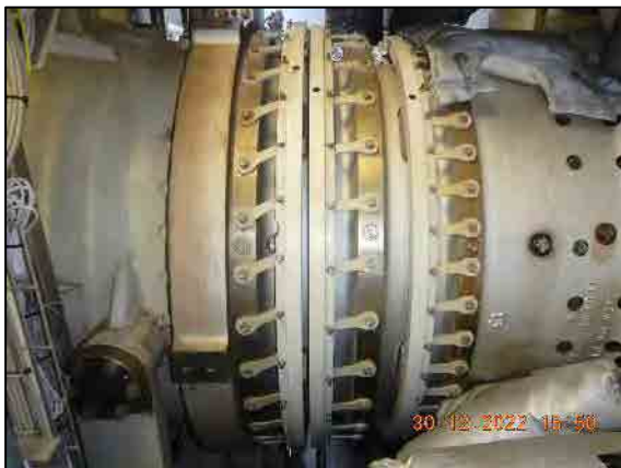
GV arms and lever mechanism on right side.
