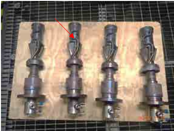
Dismantled burner#15 overall condition.
