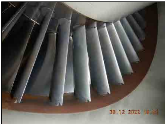
Compressor Inlet guide vanes stage 0.
