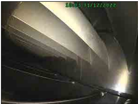
Compressor guide vanes stage 5.
