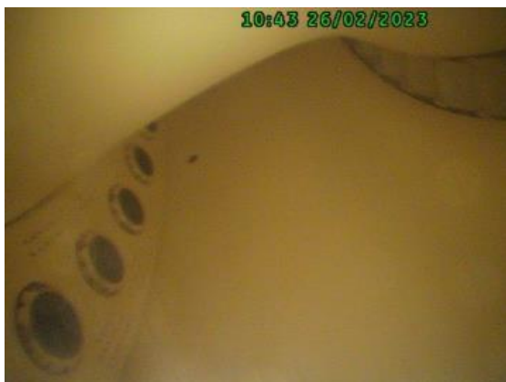
Front panel with burners from burner#15.
