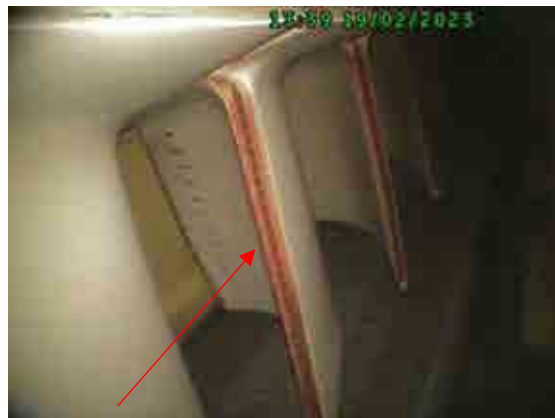
Blades 1 trailing edge cooling passage and platform.
