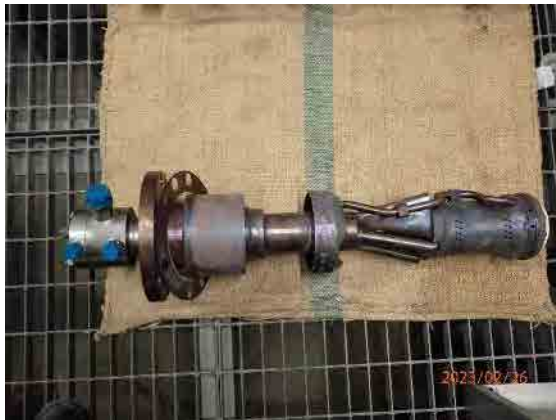
Dismantled burner#15 overall condition.
