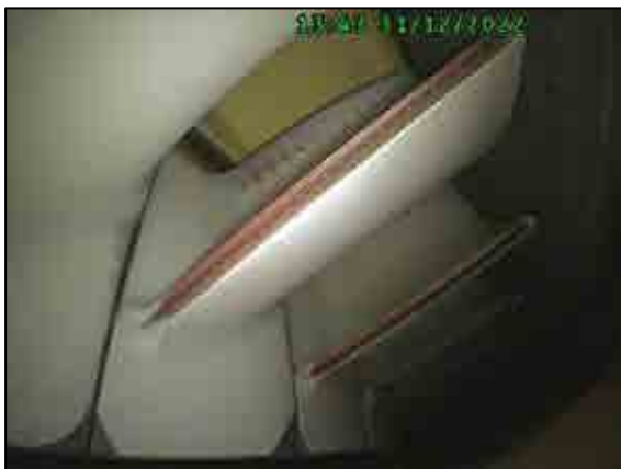
Trailing edge cooling passages of turbine blades 1.
