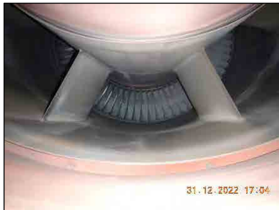
Inner/outer heatshields and struts at bottom area.
