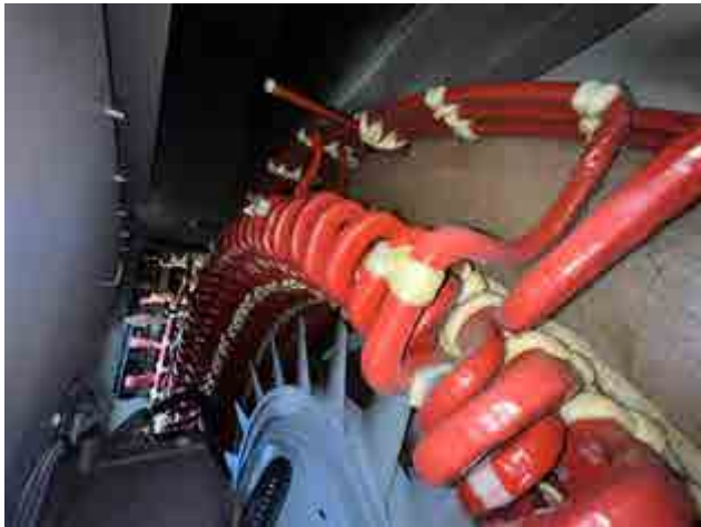
6 Stator winding 3
