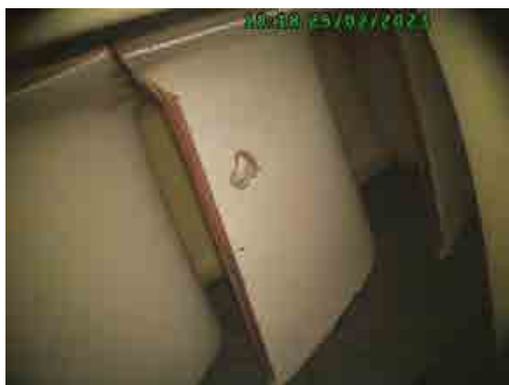
Observed TBC loss on Turbine blades 1 trailing edge.
