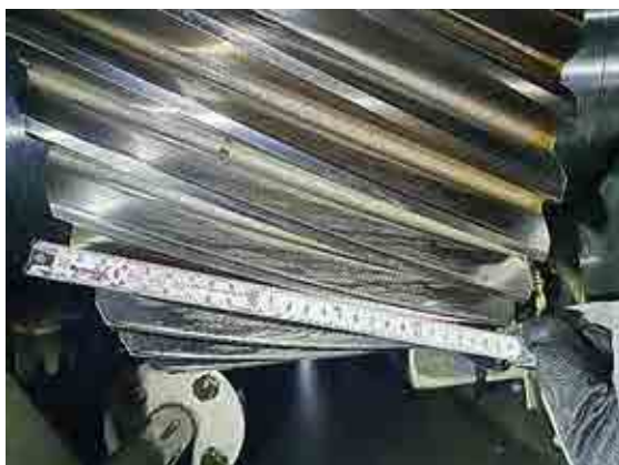
White mark on pinion gear generator side.
