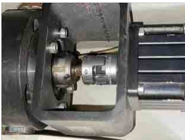
3 VGV motor coupling was gone.
