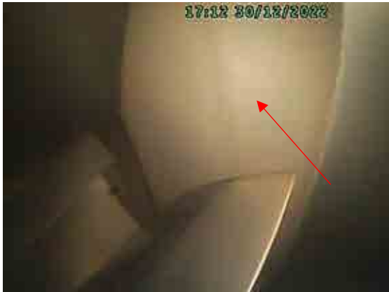
Abradable seal stage 3 condition.
