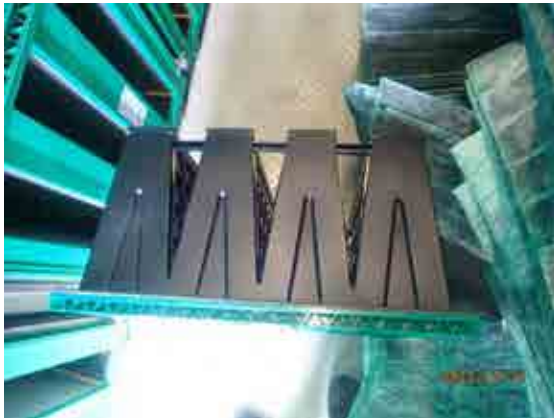
E12 fine filter as found condition.
