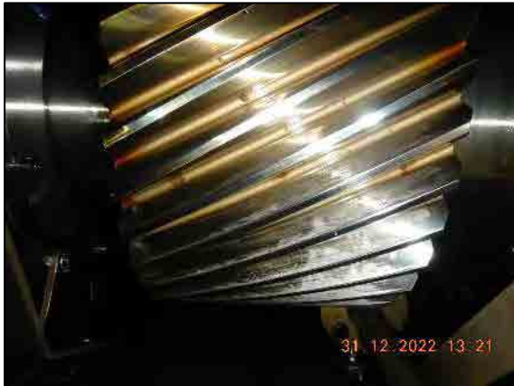
Pinion cogs active side condition (Starter motor side). Pinion cogs active side condition (Turbine side).
