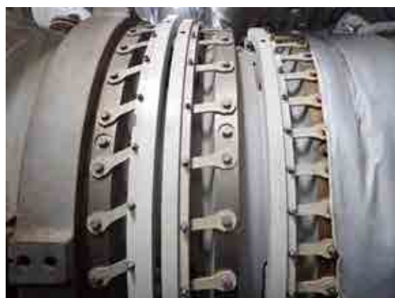
GV actuator mechanism overall condition right side.
