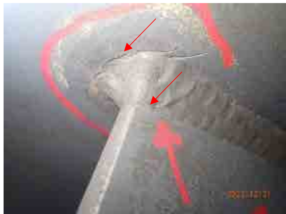
Example of crack at front support struts.
