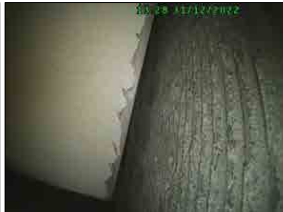
Example of turbine blade stage 1 tip condition.
