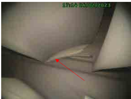
Condition leading edge tip turbine blades 3.
