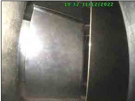
Compressor blades stage 8 condition.
