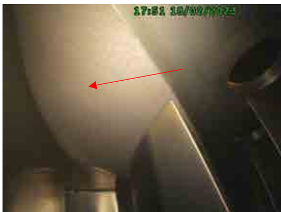
Abradable seal stage 3 condition.
