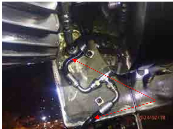
Jacking oil hose condition.
