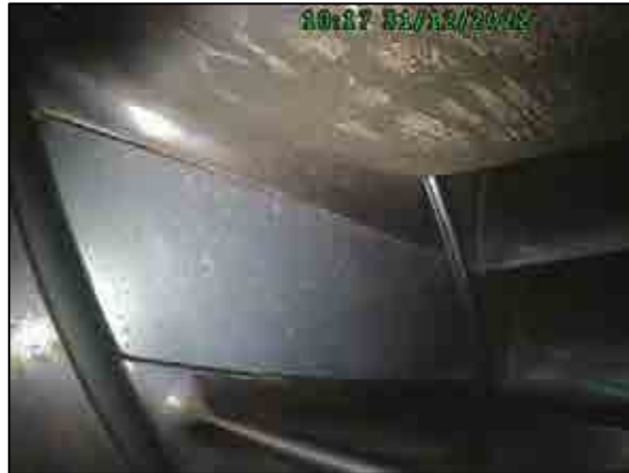
Compressor rotor stage 9 condition
