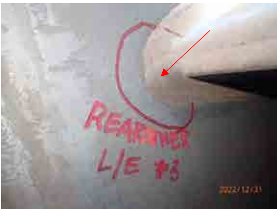
Example of crack at rear support struts.
