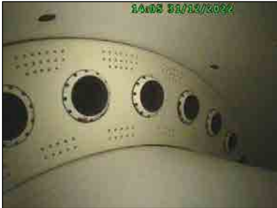
Front panel and burners tip condition.
