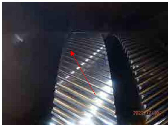
Wheel gear condition found white marks on Generator side
