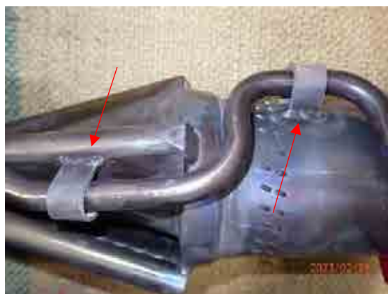
Gas fuel wings and pilot fuel pipe overall condition.
