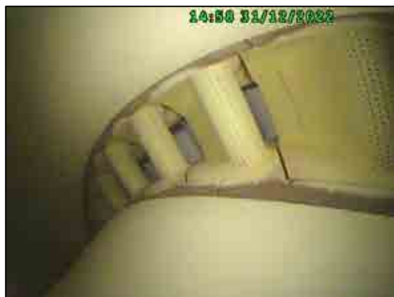
Guide vanes 1 leading edge cooling holes and inner/outer vane plates overall condition.
