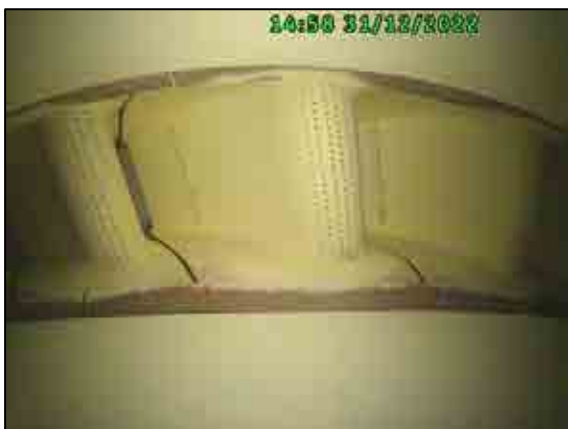
Guide vanes 1 leading edge cooling holes and inner/outer vane plates overall condition.
