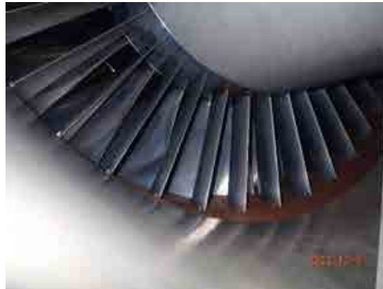
Compressor Inlet guide vanes stage 0.
