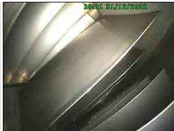
Compressor blades stage 4 condition.
