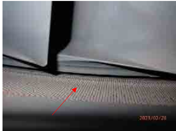
Stage 3 heat shield honeycomb overall condition.
