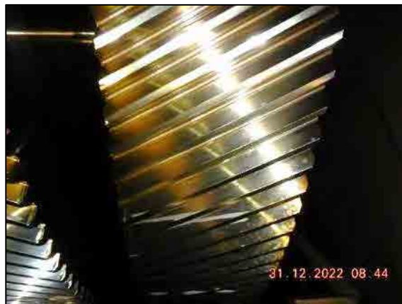
Wheel active side white mark (Turbine side).
