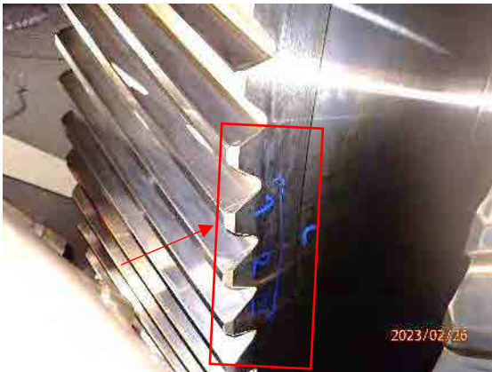
Electro static discharge 15 cm at left and right side on right wheel and follow up location at next inspection
