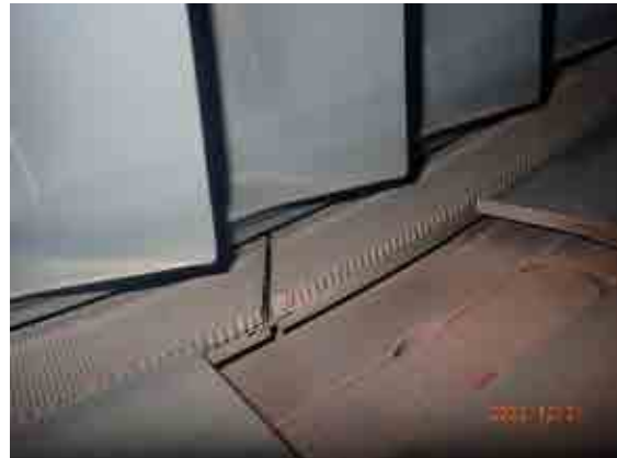
Blade 3 tip with honeycomb condition.
