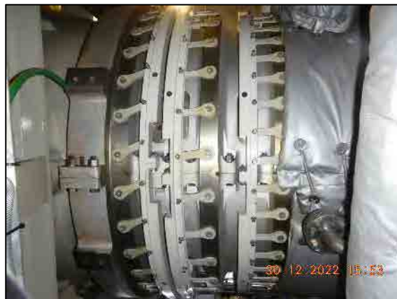
GV arms and lever mechanism at bottom.
