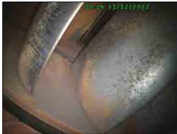
Compressor guide vanes stage 12.
