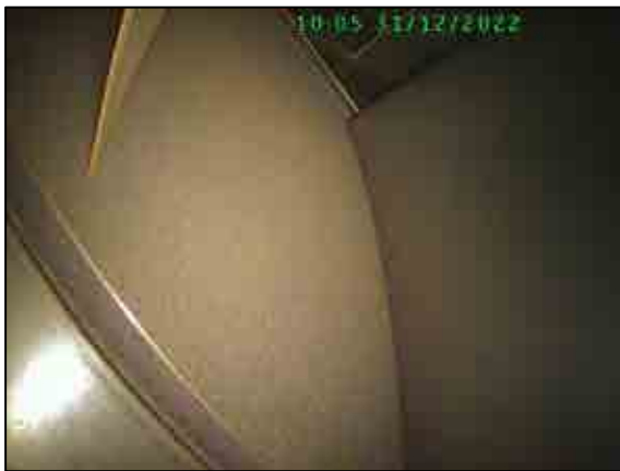
Abradable seal stage 5 condition.
