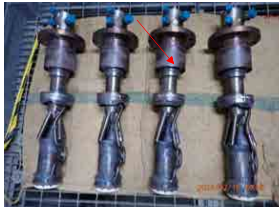
Dismantled burner#7 overall condition.
