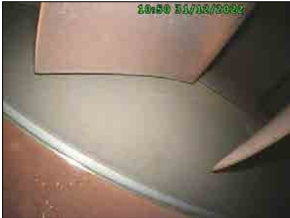
Abradable seal stage 14 condition.
