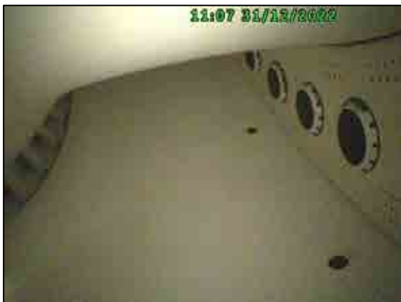
Inner/outer wall TBC overall condition.
