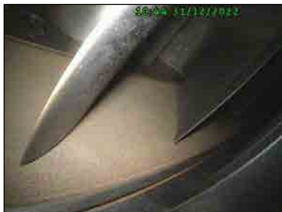
Abradable seal stage 12 condition.
