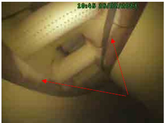
Inner/Outer vane plate condition at burner position 15.
