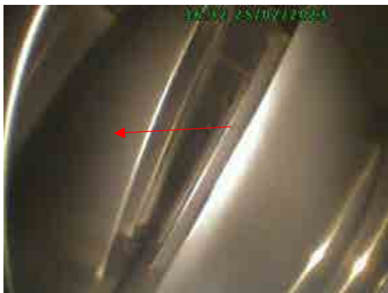
Compressor blades stage 3 condition.
