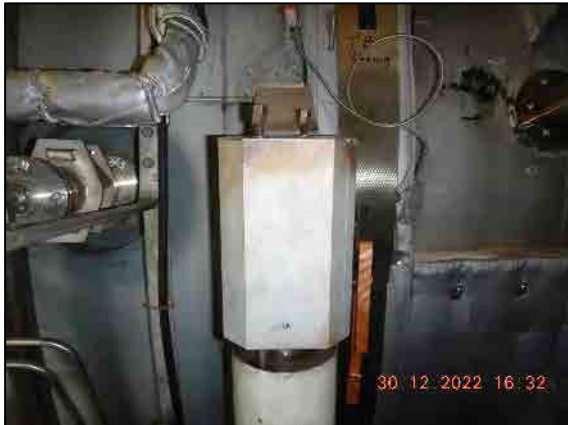
Right central casing support pendulum.
