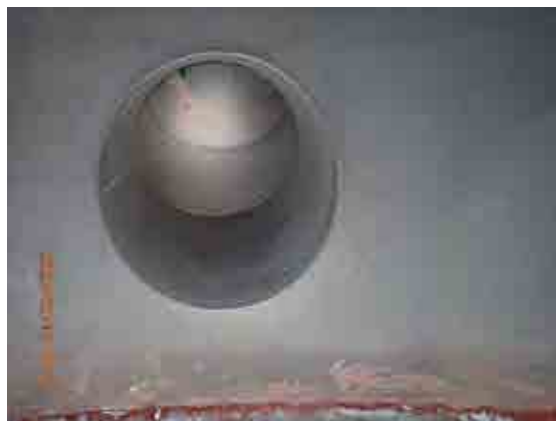
Bleed pipe left hole condition.
