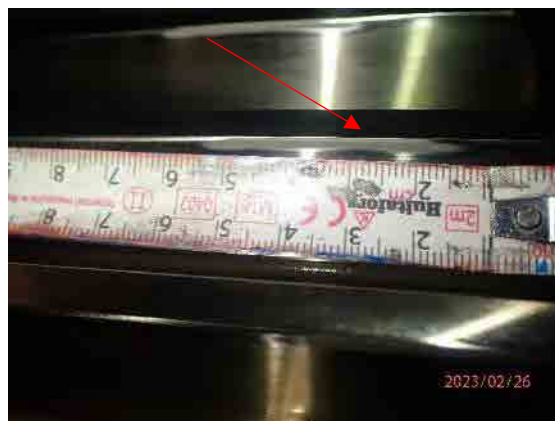
White mark 40 mm at right side on right wheel.
