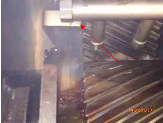
Oil leakage on left side of manifold.
