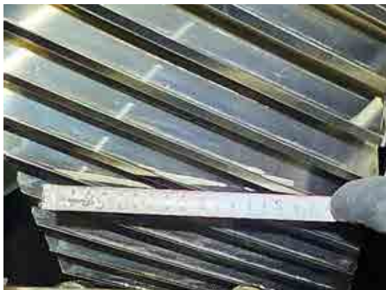
Electro discharge 16 cm at left side on left wheel and follow up location at next inspection.
