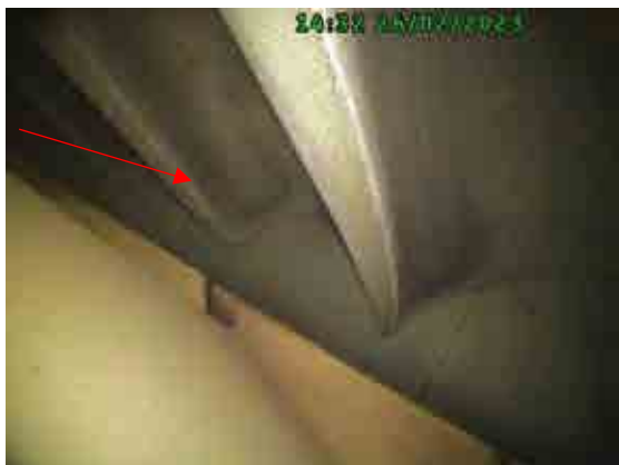
Turbine blades 2 leading edge condition.
