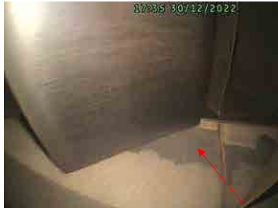
Abradable seal stage 8 condition.
